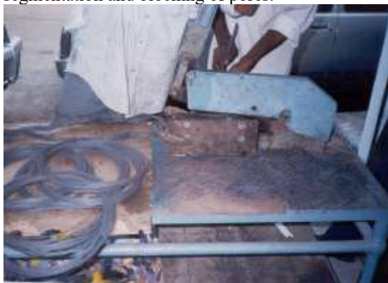
Fig 1.8.1 Chopping the steel fibre with shear cutting machine.
