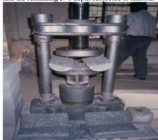
Fig 3.5.2 Split tensile strength for cylinders
