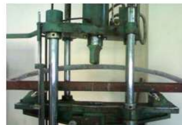
Fig. 6 Load applying on GFRP Leaf spring
