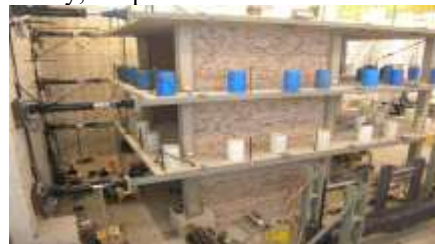
Figure 1 : Test Structure with Infill Walls
