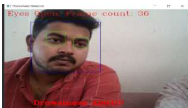
Figure 4: Test score when eye is open
